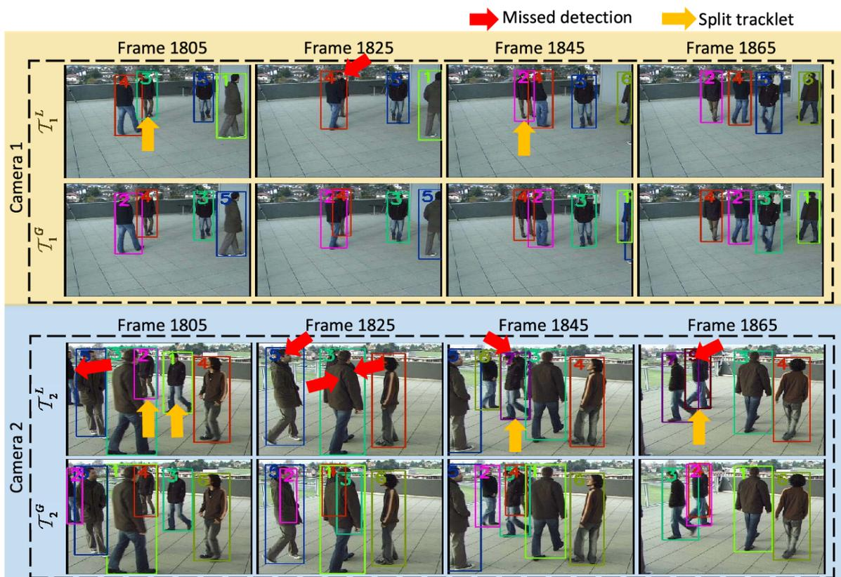
Figura 9 – Multi-Target Multi-Camera Tracking by Tracklet-to-Target Assignment. (HE et al., 2020)
